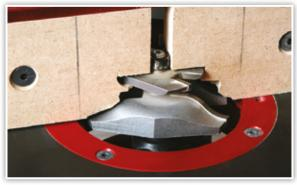
Reduce the fence opening as much as possible in order to provide support for the work-piece. When using large diameter bits, such as a raised panel bit, make a zero-clearance fence opening.
