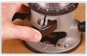
Secure the router motor in the base before plugging it in to the power outlet.
