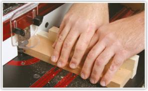
Use a jig or miter gauge when shaping end of narrow stock.
