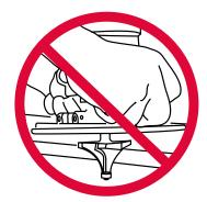
**5.** Never use a large diameter bit in a handheld router. Refer to Amana Tool® website and catalog for guidelines.
