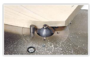
Use a starting pin when shaping curved stock without the use of a template.
