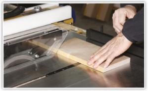
17. Allow saw to reach maximum RPM before starting the cut.
