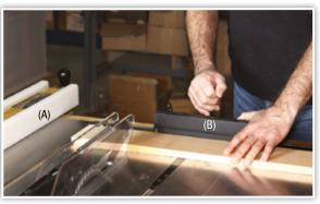
19. Never use fence(A) and the guide(B) at the same time. Do not force the blade into the cut. Use a feed rate that does not bog down the saw.
