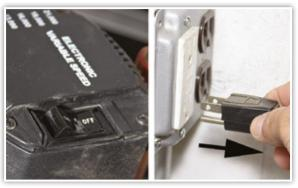
Make certain that the power switch is in the "OFF" position before connecting the router to the power source.
