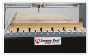
**7.** Remove all tools and set-up gauges from the table before powering up your machine.
