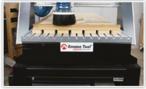
**25.** Dust collection system and vacuum systems will aid in a fires speed travel. A tool left running in the same place for a sufficient amount of time, can and will start a fire. It is essential to never leave a CNC running without an operator.
