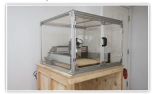
10. For smaller size CNC machines we recommend the use of an enclosure, this will not only help contain dust and noise, but will add an extra layer of safety in the event anything flying off of the machine.
