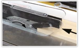
**6.** Always feed the stock against the direction of the power tool rotation.
