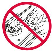
17. Avoid routing small stock. Shape a larger work-piece and then reduce it in size. If you must shape a small piece use a jig or large wooden clamp to grasp the stock.
