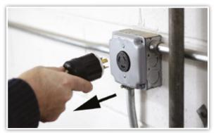
**3.** Disconnect the power tool from the power source before changing the saw blade.
