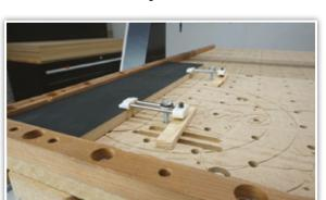
Always secure your work piece to the spoilboard using clamps, vacuum or double-sided tape. Never try to hold any work piece on the table by hand.
