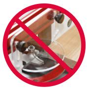
Never start the router with the router bit in contact with the stock/work-piece.  $\label{eq:contact} % \begin{subarray}{ll} \end{subarray} % \be$
