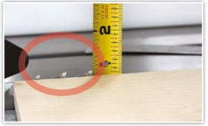
Before starting the saw, adjust the saw blade height 1/8" above the work-piece.
