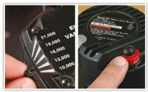
3. Never exceed the recommended RPM for the router bit. See reference chart online http://www.amanatool.com/maxrpm
