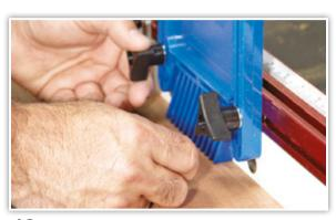
Always use featherboards to hold the work-piece firmly to the table and fence.
