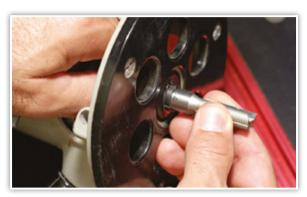
Do not bottom-out the bit in the collet; insert the bit fully and then back it out 1/8" or to stop line k, when available.
