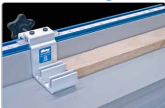
Add a stop to the fence for repeat cuts to a set depth, such as cutting tenons.
